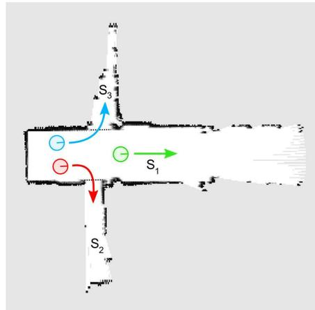
Fig. 1. Illustration of the coordination step. Robots are assigned to segments of the partial map.
